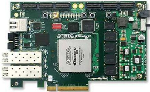
Fig. 14. FPGA evaluation board
