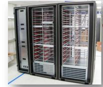
backplanes connected with copper cables in a group: "Black Network"
