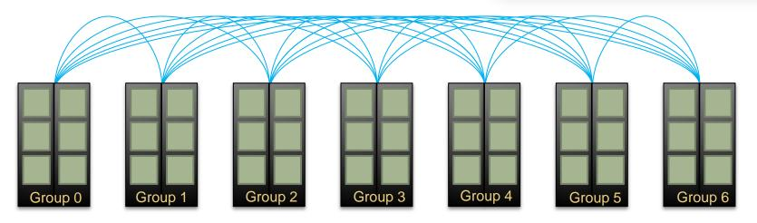
*Example:* A 7-group system is interconnected with 21 optical "bundles". The "bundles" can be configured between 2 or more cables wide, subject to the group limit.
