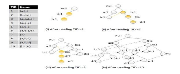
Fig. 7. Construction of an FP-tree - Based on [28]
