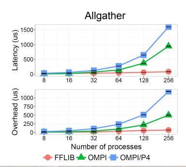
Curie, a Tier-0 system 5,040 nodes 2 eight-core Intel Sandy Bridge processors Full fat-tree Infiniband QDR OMPI: Open MPI 1.8.4 OMPI/P4: Open MPI 1.8.4 + Portals 4 backend FFLIB: proof of concept library One process per computing node
