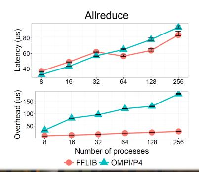
Curie, a Tier-0 system 5,040 nodes 2 eight-core Intel Sandy Bridge processors Full fat-tree Infiniband QDR OMPI: Open MPI 1.8.4 OMPI/P4: Open MPI 1.8.4 + Portals 4 backend FFLIB: proof of concept library One process per computing node More about FFLIB at http://spcl.inf.ethz.ch/Research/ Parallel\_Programming/FFlib/
