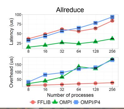
Curie, a Tier-0 system 5,040 nodes 2 eight-core Intel Sandy Bridge processors Full fat-tree Infiniband QDR OMPI: Open MPI 1.8.4 OMPI/P4: Open MPI 1.8.4 + Portals 4 backend FFLIB: proof of concept library One process per computing node
